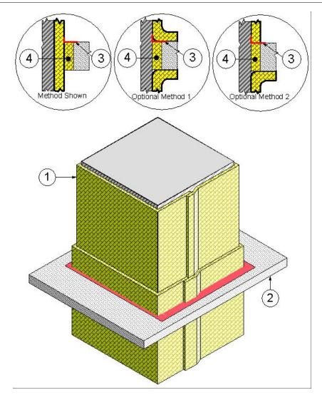
PENETRATING ITEM: An airtight duct system with vertical duct sections constructed of min. 26 GA (0.0179 in) plain sheet steel with max. 1296-in. area and max. 54-in. width (max. dim. 24-in. x max. 54-in.) and insulated with 1 layer of 6 pcf, 1-1/2 in. Unifrax Corporation's FyreWrap EZ 1.5 Duct Insulation as detailed in Design VAD 560 F. The FyreWrap EZ 1.5 Duct Insulation was run continuously through the floor/ceiling assembly (Item 2).
