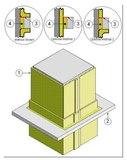
1. PENETRATING ITEM: A continuously welded, liquidtight L-shaped duct system with horizontal and vertical duct sections constructed of minimum 16 GA (0.028 in.) plain sheet steel or 18 GA stainless steel with max. 2704-in. area and max. 52-in. width (max. dim. 52-in. x max. 52-in.) and insulated with 1 layer of 6 pcf, 1-1/2 in. Unifrax Corporation's FyreWrap EZ 1.5 Duct Insulation as detailed in as detailed
