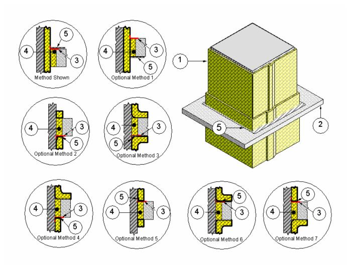
1. PENETRATING ITEM: An airtight duct system with vertical duct sections constructed of min. 26 GA (0.0179 in) plain sheet steel with max. 1296-in. area
