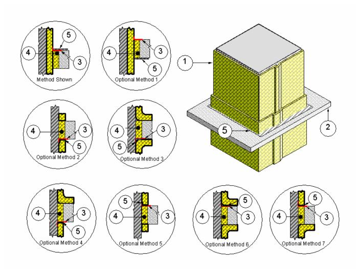
1. PENETRATING ITEM: An airtight duct system with vertical duct sections constructed of min. 26 GA (0.0179 in) plain sheet steel with max. 1296-in. area and max. 54-in. width (max. dim. 24-in. x max. 54-in.) and insulated with 1 layer of 6 pcf, 1-1/2 in. Unifrax Corporation's FyreWrap EZ
