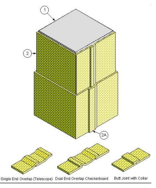
1. VENTILATION DUCT: An airtight duct system with vertical duct sections constructed of min. 26 GA (0.0179 in.) plain sheet steel with a max. 1296-in. area and a max. 54-in. width (max. 24-in. high x max. 54-in. wide). When required, equip the duct with a field fabricated
