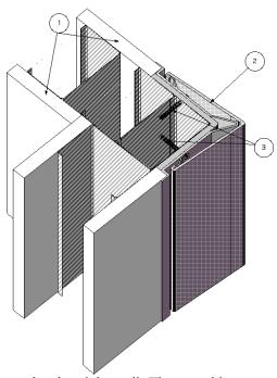
height of the wall. The assembly consists of a flexible insulative mat material with a steel cover angle, an extruded Class A (I) polyvinyl chloride (PVC) retainer or an extruded aluminum retainer with a built in shock cushion and a high impact extruded polyvinyl chloride (PVC) cover.
