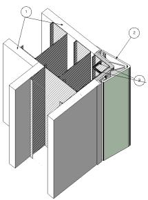
chloride (PVC) retainer or an extruded aluminum retainer with a built in shock cushion and a high impact extruded polyvinyl chloride (PVC) cover.
