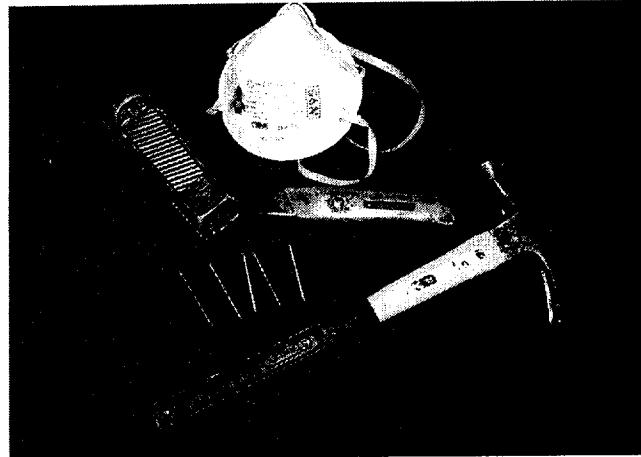
**Review the attached multiple page MATERIAL SAFETY DATA SHEET (MSDS) regarding the safe handling of the gasket material. Be sure to utilize the specified 3M or equivalent air purifying respirator while handling and fabricating this material. All trimming or cutting must be done outdoors and NOT in a closed area or indoors.**
