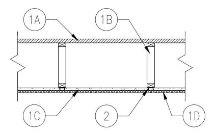
FLOOR/CEILING ASSEMBLY: Use a 1 hour fire-rated floor/ceiling constructed in accordance with material and construction specifications of UL Design No. L585 and with min. requirements as specified below:
