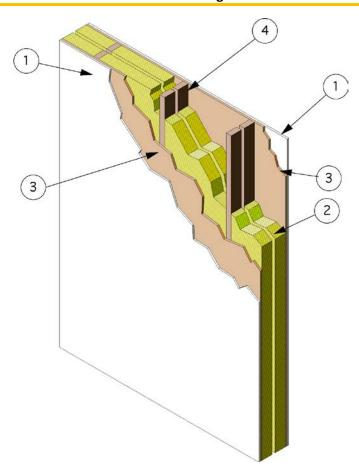
1. WALLBOARD, GYPSUM: One layer 5/8 in. thick x 4 ft. x 10 ft. Type X gypsum wallboard, applied vertically over the panels to each side of the assembly, fastened through the panels with 8d cement coated nails, 2-3/8 in. long, cup-head drywall nails with 0.113 in. shank diameter and 9/32 in. head diameter, spaced 8 in. on center (oc) along all studs and runners.
