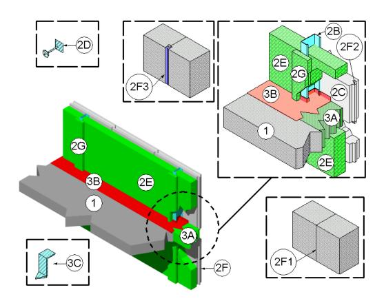
CONCRETE FLOOR ASSEMBLY: Twohour rated concrete floor assembly made from either lightweight or normal weight concrete with a density of 100 to 150 pcf, having a minimum thickness of 4-1/2" at the joint face. When a longitudinal recess (blockout) is required to contain an architectural joint system, increase concrete floor assembly thickness to maintain a minimum thickness of 4-1/2" and accommodate
