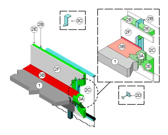
CONCRETE FLOOR ASSEMBLY: Twohour rated concrete floor assembly made from either lightweight or normal weight concrete with a density of 100 to 150 pcf, having a minimum thickness of 4-1/2" at the joint face. When a longitudinal recess (blockout) is required to contain an architectural joint system, increase concrete floor assembly thickness to maintain a minimum
