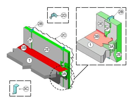
CONCRETE FLOOR ASSEMBLY: Two-hour rated concrete floor assembly made from either lightweight or normal weight concrete with a density of 100 to 150 pcf, having a minimum thickness of 4-1/2" at the joint face. When a longitudinal recess (blockout) is required to contain an architectural joint system,
