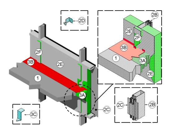
CONCRETE FLOOR ASSEMBLY: Twohour rated concrete floor assembly made from either lightweight or normal weight concrete with a density of 100 to 150 pcf, having a minimum thickness of 4-1/2" at the joint face. When a longitudinal recess (blockout) is required
