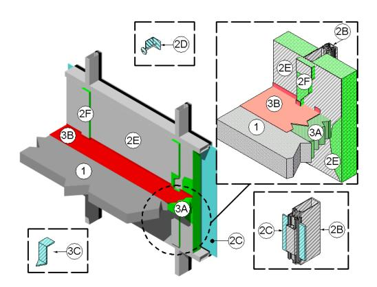
CONCRETE FLOOR ASSEMBLY: Twohour rated concrete floor assembly made from either lightweight or normal weight concrete with a density of 100 to 150 pcf, having a minimum thickness of 4-1/2" at the joint face. When a longitudinal recess (blockout) is required to contain an architectural joint system, increase concrete floor assembly thickness to maintain a minimum thickness of 4-1/2" and accommodate depth of blockout formed in the concrete: blockout width unrestricted.
