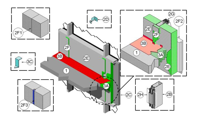
CONCRETE FLOOR ASSEMBLY: Twohour rated concrete floor assembly made from either lightweight or normal weight concrete with a density of 100 to 150 pcf, having a minimum thickness of 4-1/2" at the joint face. When a longitudinal recess (blockout) is required
