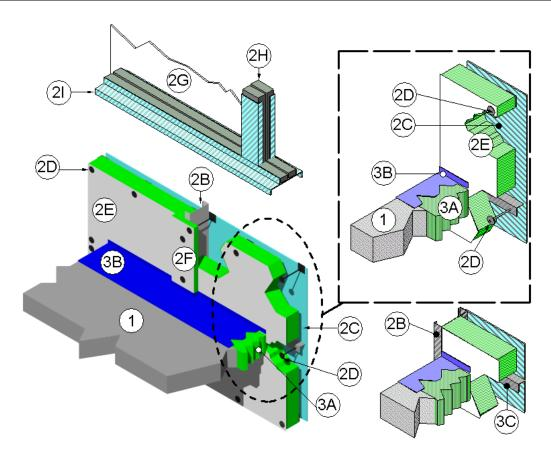
CONCRETE FLOOR ASSEMBLY: Three-hour rated concrete floor assembly made from either lightweight or normal weight concrete with a density of 100 to 150 pcf, having a minimum thickness of 4-1/2" at the joint face. When a longitudinal recess (blockout) is required to contain an architectural joint
