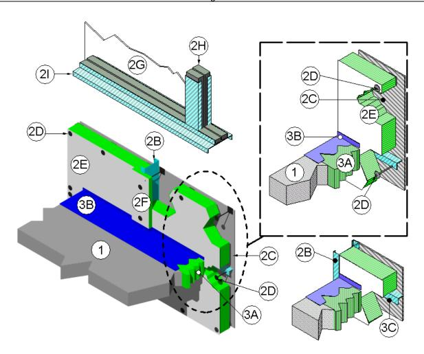
CONCRETE FLOOR ASSEMBLY: Two-hour rated concrete floor assembly made from either lightweight or normal weight concrete with a density of 100 to 150 pcf, having a minimum thickness of 4-1/2" at the joint face. When a longitudinal recess (blockout) is required
