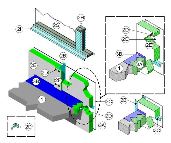
CONCRETE FLOOR ASSEMBLY: Three-hour rated concrete floor assembly made from either lightweight or normal weight concrete with a density of 100 to 150 pcf, having a minimum thickness of 4-1/2" at the joint face. When a longitudinal recess (blockout) is required to contain an architectural joint system, increase concrete floor assembly thickness to maintain a minimum thickness of 4-1/2" and accommodate depth of blockout formed in the concrete: blockout width unrestricted.
