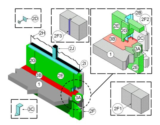
CONCRETE FLOOR ASSEMBLY: Twohour rated concrete floor assembly made from either lightweight or normal weight concrete with a density of 100 to 150 pcf, having a minimum thickness of 4-1/2 in. at the joint face. When a longitudinal recess (blockout) is required to contain an architectural joint system, increase concrete floor assembly thickness to maintain a minimum thickness of 4-1/2 in. and accommodate depth of blockout formed in the concrete: blockout width unrestricted.
