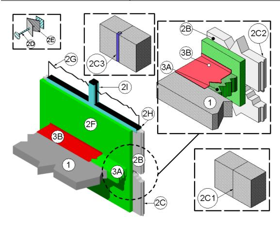
CONCRETE FLOOR ASSEMBLY: Two-hour rated concrete floor assembly made from either lightweight or normal weight concrete with a density of 100 to 150 pcf, having a minimum thickness of 4-1/2 in. at the joint face. When a longitudinal recess (blockout) is required
