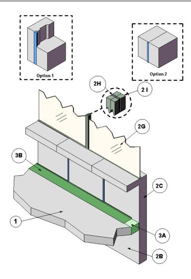
1. CONCRETE FLOOR ASSEMBLY: Three-hour rated concrete floor assembly made from either lightweight or normal weight concrete with a density of 100 to 150 pcf, having a min. thickness of 5.7 in. at the joint face. When a longitudinal recess (blockout)
