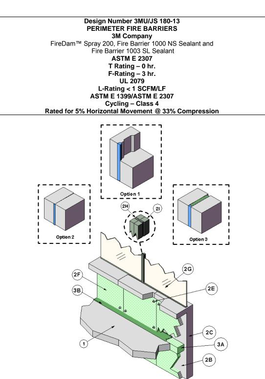
CONCRETE FLOOR ASSEMBLY: Threehour rated concrete floor assembly made from either lightweight or normal weight concrete with a density of 100 to 150 pcf, having a minimum thickness of 5.7 inches at the joint face. When a longitudinal
