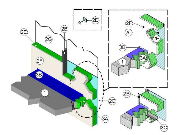
CONCRETE FLOOR ASSEMBLY: Twohour rated concrete floor assembly made from either lightweight or normal weight concrete with a density of 100 to 150 pcf, having a minimum thickness of 4-1/2" at the joint face. When a
