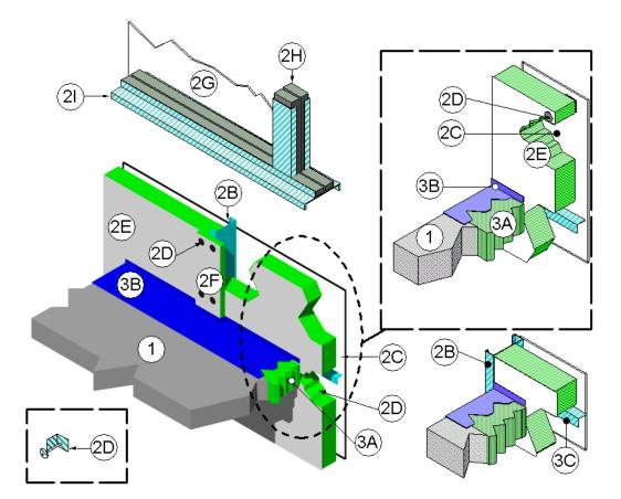
CONCRETE FLOOR ASSEMBLY: Three-hour rated concrete floor assembly made from either lightweight or normal weight concrete with a density of 100 to 150 pcf, having a minimum thickness of 4-1/2" at the joint face. When a longitudinal recess (blockout) is
