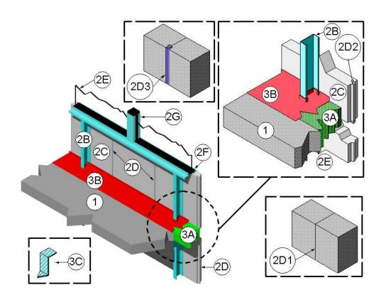
CONCRETE FLOOR ASSEMBLY: Two-hour rated concrete floor assembly made from either lightweight or normal weight concrete with a density of 100 to 150 pcf, having a minimum thickness of 4-1/2 in. at the joint face. When a longitudinal recess (blockout) is required
