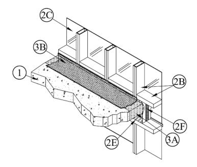
1. CONCRETE FLOOR ASSEMBLY: 3-hr rated concrete floor assembly made from either lightweight or normal weight concrete with a density of 100 to 150 pcf, having a min. thickness of 4-1/2 in. at the joint face. When a longitudinal recess (blockout) is required to contain an architectural joint system, increase concrete floor assembly thickness to maintain a min. thickness of 4-1/2 in. and accommodate
