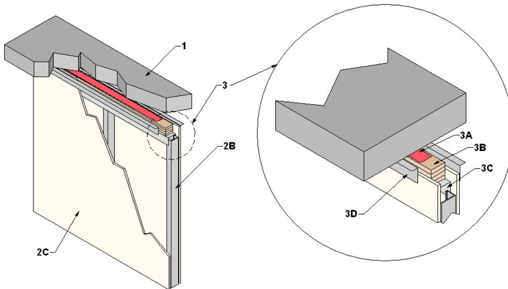
1. **FLOOR ASSEMBLY:** Normal weight concrete floor assembly with a minimum 1 hr fire resistance.
