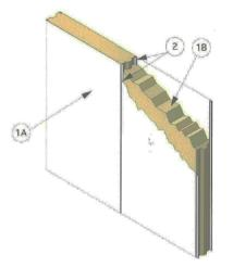
**1. INSULATED WALL PANELS:** Steel-faced panels, with a core of mineral wool insulation
