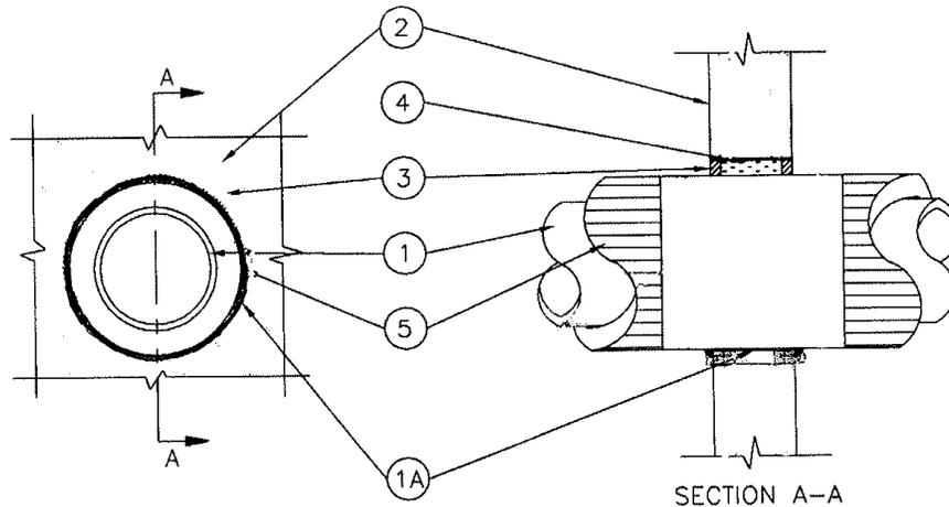
**1. PENETRATING ITEM:** See Table 1 below for approved penetrating items. Single penetrations only, max. hole size and annular space not to exceed dimensions stated in the table.
