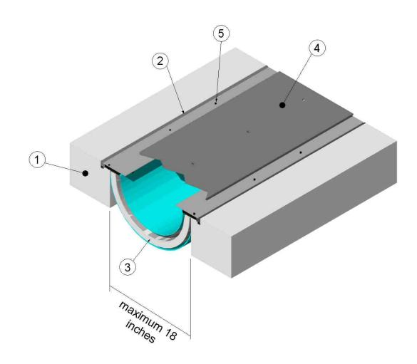
CONCRETE FLOOR ASSEMBLY: Construct a two-hour-rated concrete floor assembly made from either lightweight or normal weight concrete with a density of 100 - 150 pounds per cubic foot, with a minimum thickness of 4-1/2 inches at the joint face. When a longitudinal recess (blockout) is required to contain an architectural joint system, increase concrete floor assembly
