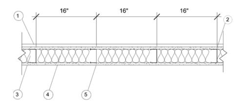
**1. POLYPROPYLENE SIDING:** Ply Gem Residential Solutions polypropylene siding products are molded, polypropylene (PP) siding.
