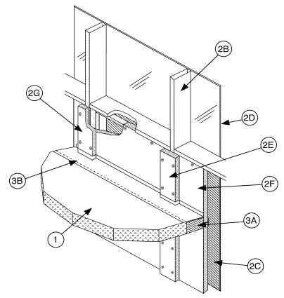
1. FLOOR ASSEMBLY: Two-hour rated concrete floor assembly made from either lightweight or normal weight concrete with a density of 100-150 pcf, with a min. thickness of 4-1/2-in. at the joint face. Overall slab thickness may increase to accommodate various blockout depths (longitudinal recesses) formed in the concrete, to house an architectural cover plate. The blockout width may also vary without restriction.
