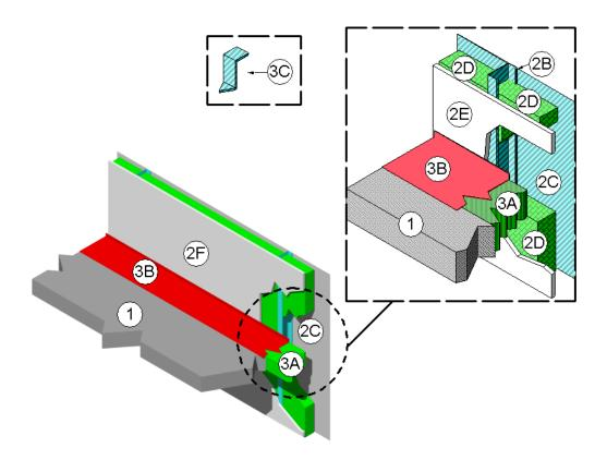
CONCRETE FLOOR ASSEMBLY: Two hour rated concrete floor assembly made from either lightweight or normal weight concrete with a density of 100 to 150 pcf, having a minimum thickness of 4-1/2 in. at the joint face. When a longitudinal recess (blockout) is required to contain an architectural joint system, increase concrete floor assembly thickness to maintain a minimum thickness of 4-1/2 in. and accommodate depth of blockout formed in the concrete: blockout width unrestricted.
