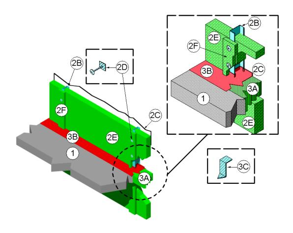
CONCRETE FLOOR ASSEMBLY: Two hour rated concrete floor assembly made from either lightweight or normal weight concrete with a density of 100 to 150 pcf, having a minimum thickness of 4-1/2 in. at the joint face. When a longitudinal recess (blockout) is required to contain an architectural joint system, increase concrete floor assembly thickness to maintain a minimum thickness of 4-1/2 in. and accommodate
