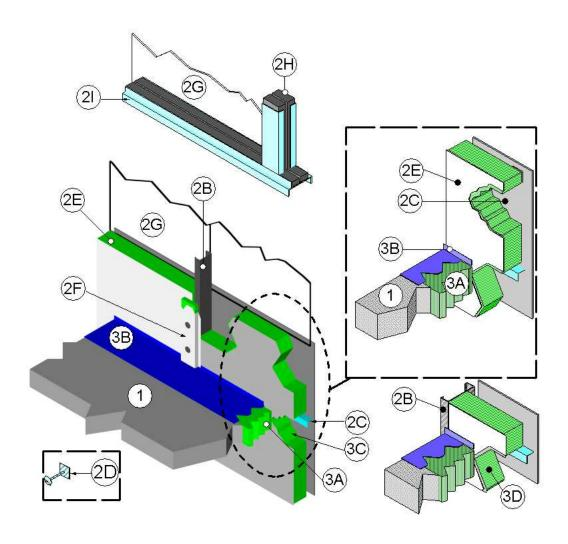
CONCRETE FLOOR ASSEMBLY: Two hour rated concrete floor assembly made from either lightweight or normal weight concrete with a density of 100 to
