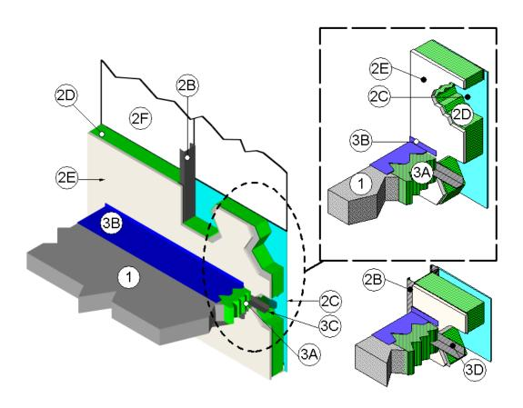
CONCRETE FLOOR ASSEMBLY: Two hour rated concrete floor assembly made from either lightweight or normal weight concrete with a density of 100 to 150 pcf, having a minimum thickness of 4-1/2 in. at the joint face. When a longitudinal recess (blockout) is required to contain an architectural joint
