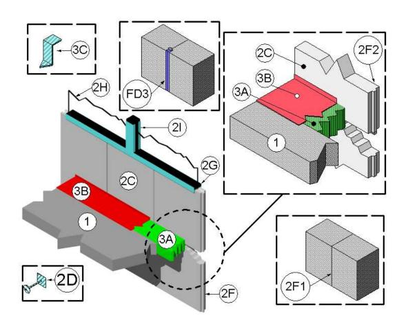
CONCRETE FLOOR ASSEMBLY: Two hour rated concrete floor assembly made from either lightweight or normal weight concrete with a density of 100 to 150 pcf, having a minimum thickness of 4-1/2 in. at the joint face. When a longitudinal recess (blockout) is required to contain an architectural joint system, increase concrete floor assembly thickness to maintain a minimum thickness of 4-1/2 in. and accommodate
