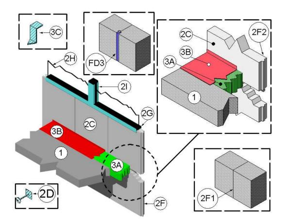
CONCRETE FLOOR ASSEMBLY: Two hour rated concrete floor assembly made from either lightweight or normal weight concrete with a density of 100 to 150 pcf, having a minimum thickness of 4-1/2 in. at the joint face. When a
