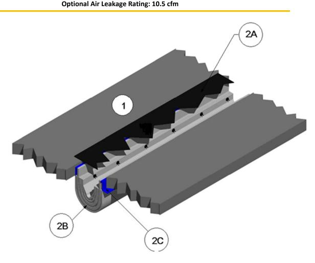
1. CONCRETE FLOOR ASSEMBLY: While conforming to the fire resistance rating requirements, the overall slab thickness may vary to accommodate various blockout depths (longitudinal recesses) formed in the concrete, to house the architectural joint system, or to conform to the requirements relative to the fire barrier thickness and joint width in accordance
