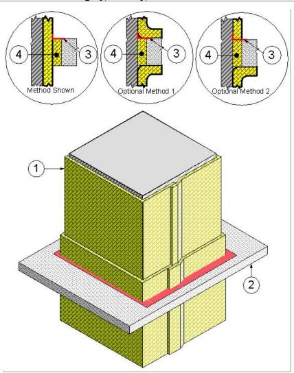
1. PENETRATING ITEM: An airtight duct system with vertical duct sections constructed of min. 26 GA (0.0179 in) plain sheet steel with max. 1296-in. area and max. 54-in. width (max. dim. 24-in. x max. 54-in.) and insulated as detailed in Design VAD 560 F.
