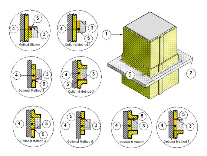
PENETRATING ITEM: An airtight duct system with vertical duct sections constructed of min. 26 GA (0.0179 in) plain sheet steel with max. 1296-in. area and max. 54-in. width (max. dim. 24-in. x max. 54-in.) and insulated as detailed in Design VAD 560 F.
