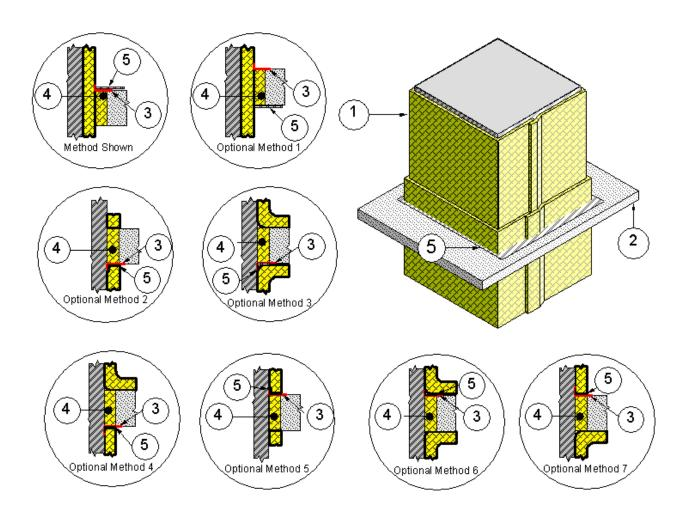
1. PENETRATING ITEM: An airtight duct system with vertical duct sections constructed of min. 26 GA (0.0179 in) plain sheet steel with max. 1296-in. area and max. 54-in. width (max. dim. 24-in. x max. 54-in.) and insulated as detailed in Design VAD 560 F.
