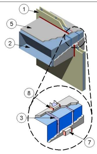
1. GYPSUM WALL ASSEMBLY: Construct a nominal 6-1/8-inch deep, two-hour rated wall assembly using minimum 25-gauge, 3-5/8-inch deep with 1-1/4-inch legs, steel studs spaced maximum 24 inches on center (o.c.). Secure studs with minimum #6 x 3/8-inch steel stud framing screws to 25-gauge steel, channel-shaped, floor and ceiling runners measuring 1/2-inch high by 3-5/8-inch deep. Secure floor and ceiling
