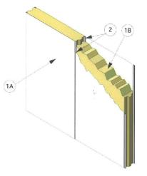
**1. INSULATED WALL PANELS:** Steel-faced panels, with a core of mineral wool insulation
