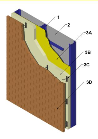
WALL FRAMING: Install nominal 3-5/8 in., 20 GA galvanized steel studs spaced 24 in. on center (oc). Secure to 20 GA top and bottom track (not shown) using 7/16 in. long pan-head framing screws. Install 16 GA CRC lateral bracing perpendicular to the steel studs spaced 48 in. oc.
