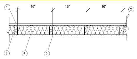
INSULATED SIDING: Westlake Royal Building Products insulated siding products are extruded, rigid polyvinyl chloride (PVC) foam backed siding.
