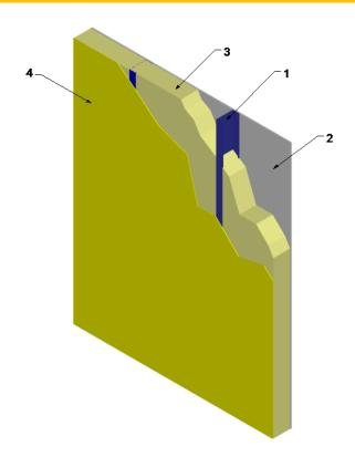
1. WALL FRAMING: Install 3-5/8 in. deep, 20 GA galvanized steel studs spaced max. 24 in. on center (oc). Secure steel studs to 3-5/8 in. 20 GA top and bottom track (not shown) using #8, 1/2 in. long, self-tapping, pan-head framing screws.
