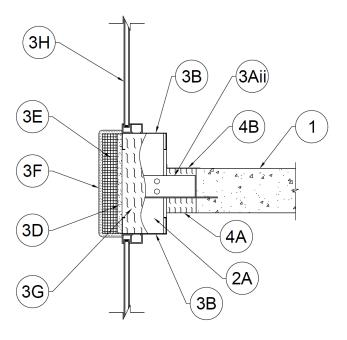
Figure 5 - Base Detail With Steel Angle Anchor
