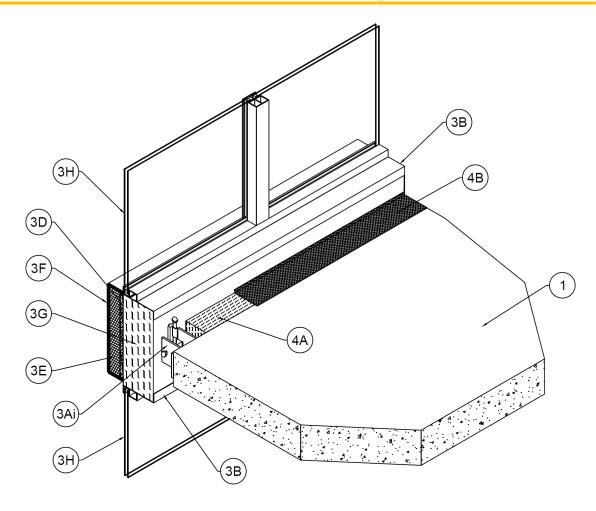
Figure 1 - Isometric with Interior Vertical Mullion Detail
