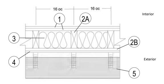
GYPSUM BOARD (Interior): Two layers Type X complying with ASTM C1396 min. 5/8 in. thick, 4 ft. wide applied vertically, fastened to framing. Face layer joints staggered with base layer and covered with paper tape and joint compound.
